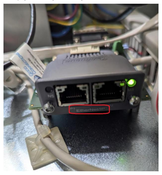
If for some reason you cannot get a camera in to the module, the module can be physically removed, but care has to be taken that power and pin alignment considerations are adhered to or the module or the host compact flash connector can be damaged.
