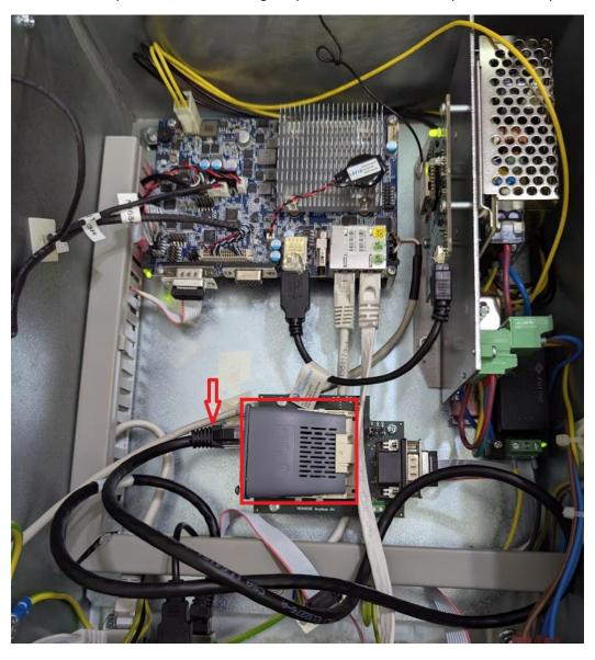
Both the Anybus M30 and M40 modules that are used by the CasTemp Wireless for Ethernet/IP will have "Ethernet/IP" printed on the faceplate similar to the picture below.
